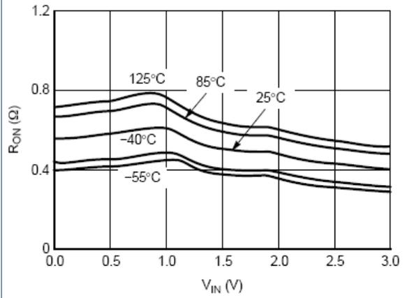
Figure 10. RON vs. VIN vs. Temperature @VCC=3.0V
