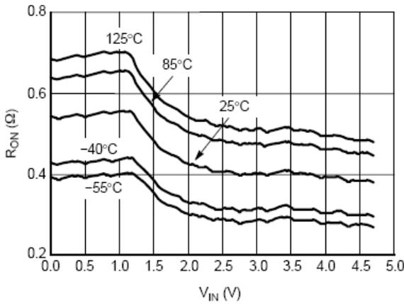
Figure 11. RON vs. VIN vs. Temperature @VCC=4.7V
