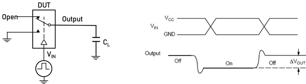
Figure 6. Charge Injection: (Q)
