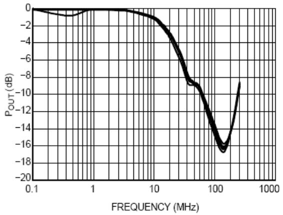
Figure 12. Bandwidth vs. Frequency @VCC=1.65V to 4.7V
