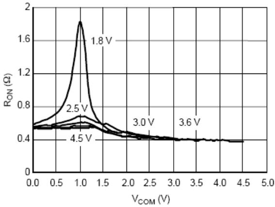
Figure 9. On-Resistance vs. COM Voltage
