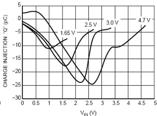
Figure 8. Charge Injection versus  $V_{IS}$
