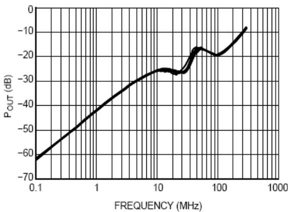
Figure 13. Off-Isolation vs. Frequency @VCC=1.65V to 4.7V
