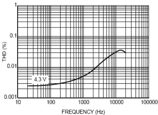
Figure 7. Total Harmonic Distortion Plus Noise Figure versus Frequency
