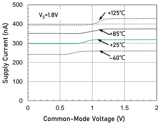
Supply Current vs. Common-Mode Input ( $V_S = 1.8\text{V}$ )
