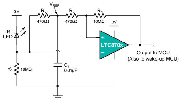
Figure 5. IR Receiver AFE Using LTC870x
