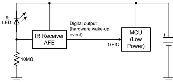
Figure 4. Coin Cell Battery Powered IR Receiver
