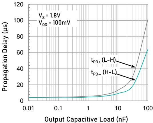
Propagation Delay vs. Capacitive Load ( $V_S = 1.8\text{V}$ )
