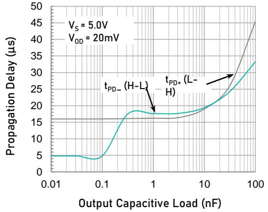
Propagation Delay vs. Capacitive Load ( $V_S = 5.0\text{V}$ )
