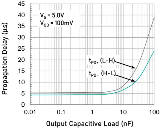
Propagation Delay vs. Capacitive Load ( $V_S = 5.0\text{V}$ )
