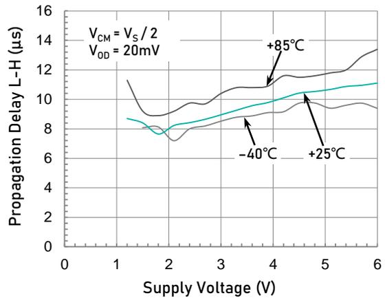
Propagation Delay L-H ( $t_{PD+}$ ) vs. Supply Voltage
