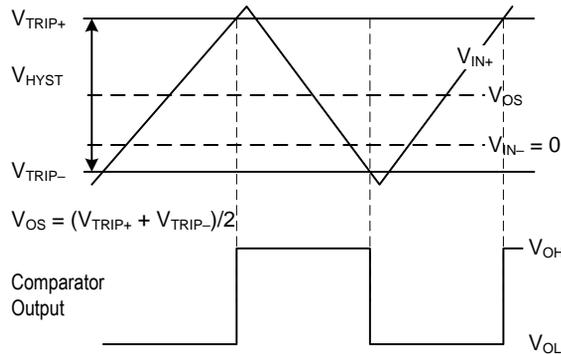
Figure 2. Input and Output Waveform, Non-inverting Input Varied
