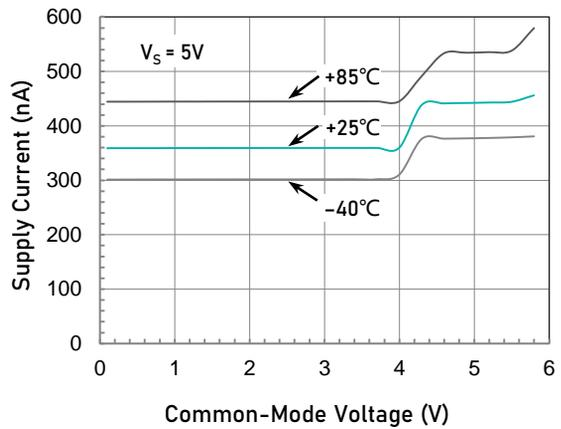
Supply Current vs. Common-Mode Input ( $V_S = 5.0\text{V}$ )
