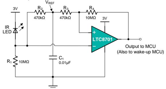
Figure 5. IR Receiver AFE Using LTC8701 (Push-Pull Output)
