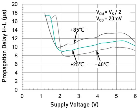
Propagation Delay H-L ( $t_{PD-}$ ) vs. Supply Voltage
