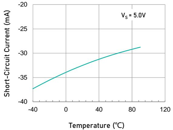
Short-Circuit Current vs. Temperature ( $V_S = 5.0\text{V}$ )
