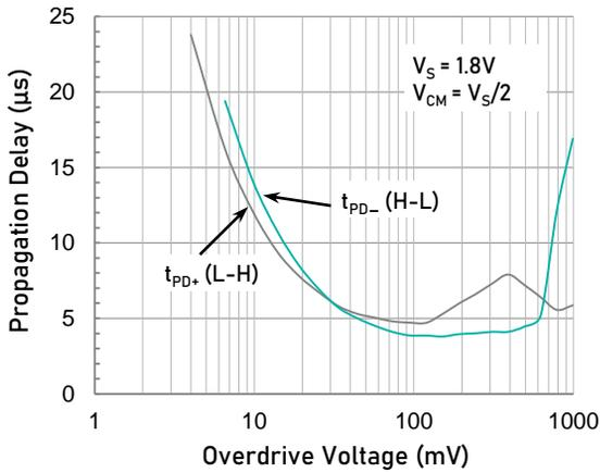
Propagation Delay vs. Input Overdrive ( $V_S = 1.8\text{V}$ )
