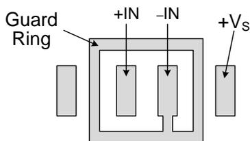
Figure 3. Use a guard ring around sensitive pins
