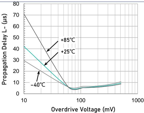
Propagation Delay H-L ( $t_{PD-}$ ) vs. Input Overdrive
