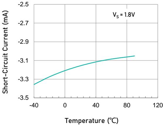
Short-Circuit Current vs. Temperature ( $V_S = 1.8\text{V}$ )
