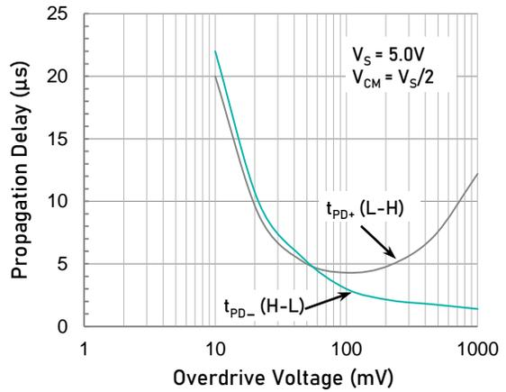
Propagation Delay vs. Input Overdrive ( $V_S = 5.0\text{V}$ )
