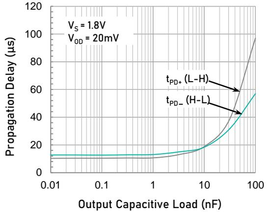
Propagation Delay vs. Capacitive Load ( $V_S = 1.8\text{V}$ )
