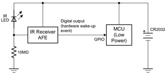
Figure 4. Coin Cell Battery Powered IR Receiver
