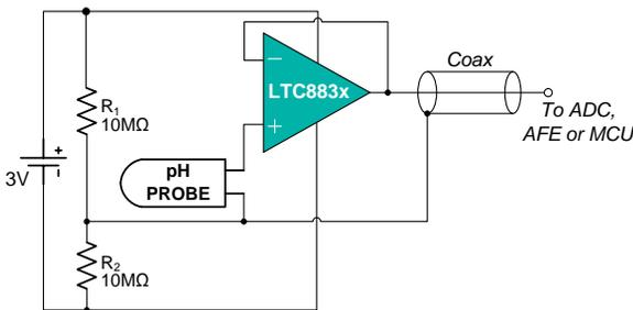
All components contained within the pH probe
