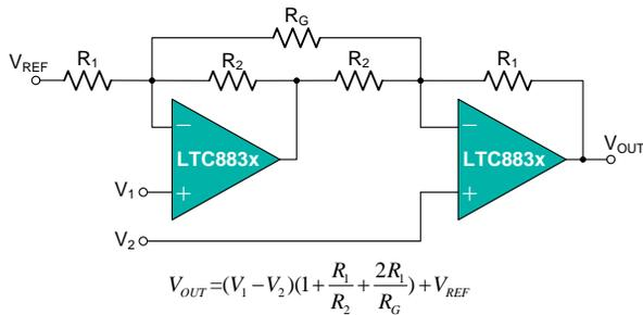
Figure 9. Instrumentation Amplifier
